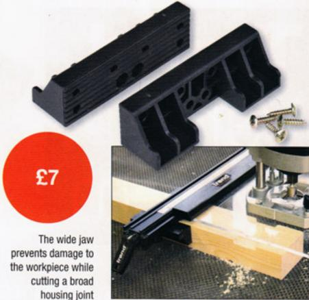
This is a pair of large smooth-faced jaws, supplied with screws to attach them to the clamp guide. To avoid clamping marks on the work being held, each jaw has six pre-drilled holes for attaching additional spreaders to increase the contact area. The jaw faces are 105mm wide and 32mm tall.
