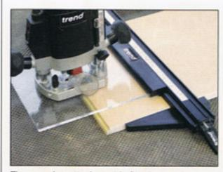
The squaring attachment is fitted to the base of the clamp guide
