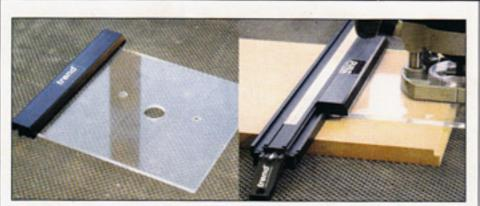
The router base plate and clamp guide allow accurate joints to be routed
