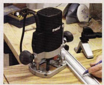
over) and a bit uncomfortable (which you may or may not be able to resolve). This is exactly the size of router that's perfect for hand-held routing. It's not too loud, and it has good low-down weight for stability and balance. The cutters are easy to change, and there's a 20mm guide bush and trammel bar attachment, plus an excellent side fence with fine adjuster.
