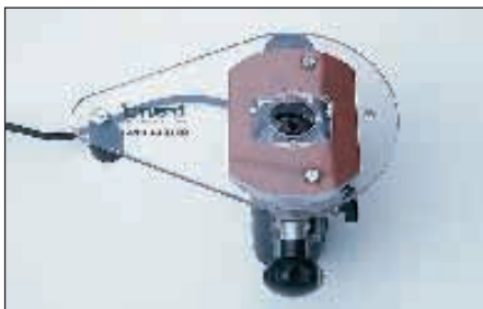
The offset base is quickly fitted to the router...
