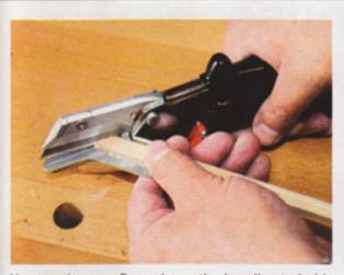
You need a very firm grip on the handles to hold the workpiece securely while you make a cut
