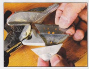
A single screw holds the replaceable Stanley knife blade in its holder
