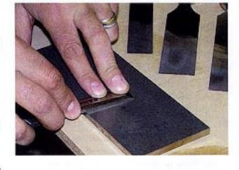
of chisels or irons that need a bit of work on the backs, now's the time to do it, breaking in the stone at the same time. But even after the stone has been broken in, the speed of the cut is very fast. Working a wire edge takes a lot less than a conventional stone.
