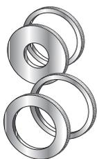
⚠ Bushing washers supplied to reduce bore diameter for certain makes and models of saw. Bushing washers must be pressed or glued into blade body of Trend 'Waveform' sawblades only. Loose bushing washers/rings must not be used.
