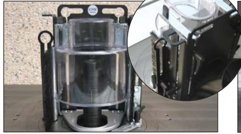
The ring fence comes as standard with the machine and replaces the back-fence when producing curved and circular work. It comes complete with adjustable guarding, lead on finger and a 100mm diameter dust extraction port.
