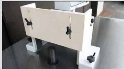
The optional tenoning hood is suitable for use with larger diameter tools (up to 300mm diameter); particularly tenon tools for producing doors.
