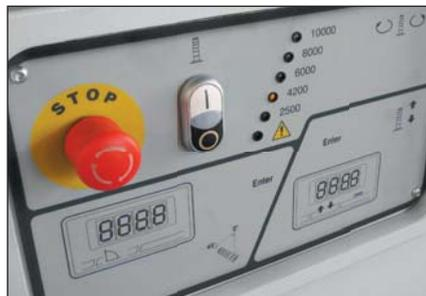
The control panel is mounted on the right-hand side of the machine and contains the soft start (automatic star, delta) button, speed indication lights and emergency stop button. The optional electronic spindle height and tilting adjustment controls would also be mounted here.
