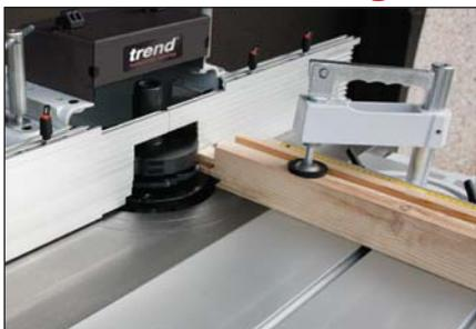
The aluminium flush mounted table runs on 8 high precision bearings ensuring smooth running and outstanding accuracy. A slot in the table is used for locating the tenoning clamp for the optional Tenoning Table.
