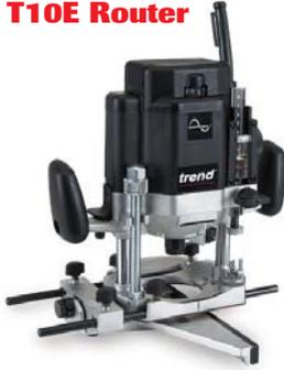
The T10E 1/2" router features a 2000 watt motor with electronic full wave variable speed and soft start, two column precision base, spindle lock for easy cutter changes, micro-adjuster parallel side-fence, precision one-piece multi-slit collet, 3-position revolving depth stop for fast settings and an adjustable inner plate for guide bush accuracy. Includes a 30mm steel guide bush, which is required for the jigs.
