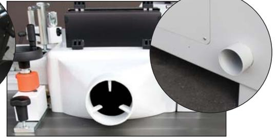
The hood has a 120mm port for dust extraction. Also a secondary 80mm outlet at the rear of the machine provides extraction from beneath the spindle.
