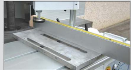
The 20mm thick tenoning table fits easily into the slot on the sliding table. Used in conjunction with the tenoning clamp and fence; suitable for getting smaller workpieces closer to the cutter heads.
