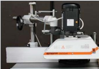
An essential piece of equipment on any spindle moulder. It provides a good finish on the material due to a constant feed speed and is the safest way to profile on a spindle moulder. It must be used with our Modular Window System. Our power feed comes complete with 3 rollers and 4 different speeds. It connects directly to a 3 phase socket on the rear of the machine. Horizontal arm is 1050mm.
