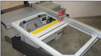
The optional table extension enables larger sections to be machined easily. Particularly suitable if you want to produce doors and larger windows.
