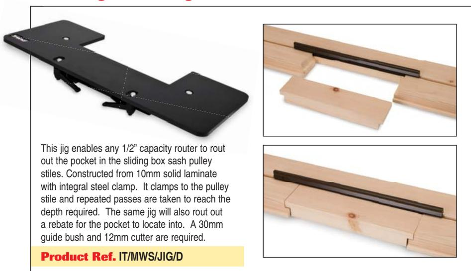
This jig enables any 1/2" capacity router to rout out the pocket in the sliding box sash pulley stiles. Constructed from 10mm solid laminate with integral steel clamp. It clamps to the pulley stile and repeated passes are taken to reach the depth required. The same jig will also rout out a rebate for the pocket to locate into. A 30mm guide bush and 12mm cutter are required.
