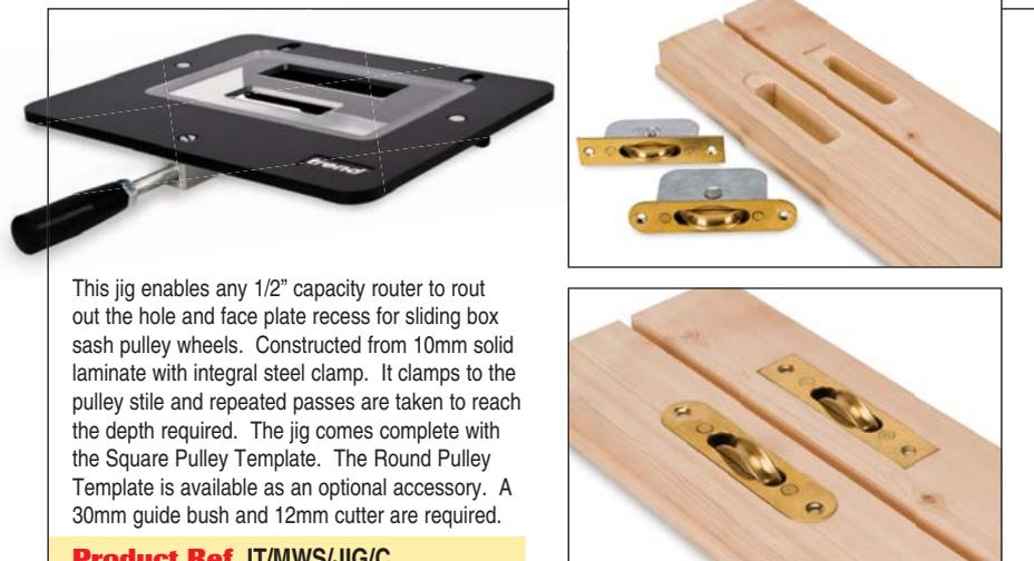
This jig enables any 1/2" capacity router to rout out the hole and face plate recess for sliding box sash pulley wheels. Constructed from 10mm solid laminate with integral steel clamp. It clamps to the pulley stile and repeated passes are taken to reach the depth required. The jig comes complete with the Square Pulley Template. The Round Pulley Template is available as an optional accessory. A 30mm guide bush and 12mm cutter are required.
