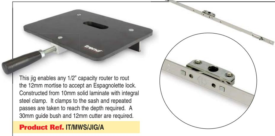
This jig enables any 1/2" capacity router to rout the 12mm mortise to accept an Espagnolette lock. Constructed from 10mm solid laminate with integral steel clamp. It clamps to the sash and repeated passes are taken to reach the depth required. A 30mm guide bush and 12mm cutter are required.
