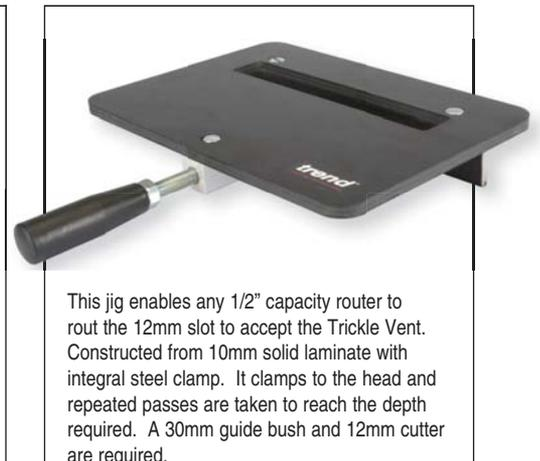
This jig enables any 1/2" capacity router to rout the 12mm slot to accept the Trickle Vent. Constructed from 10mm solid laminate with integral steel clamp. It clamps to the head and repeated passes are taken to reach the depth required. A 30mm guide bush and 12mm cutter are required.
