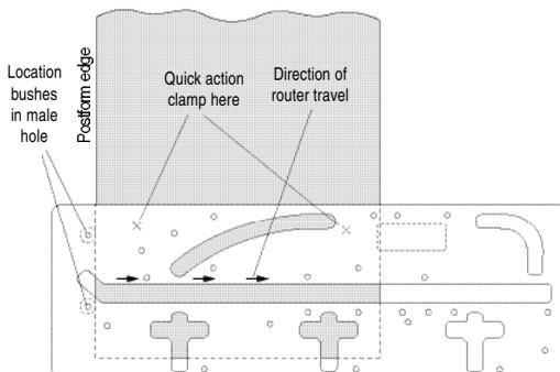
**Cutting male joint on out-of-square joints**
