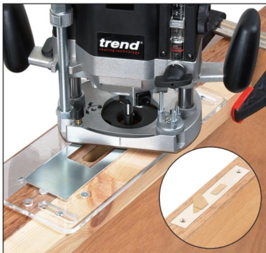
**Templates for use with any plunge router to accurately fit 2, 3 and 5 lever sash and dead mortise locks.**
