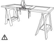
If using the jig whilst the door is hung, only a light weight router should be used. Door must be prevented from moving with wedge or similar device.
