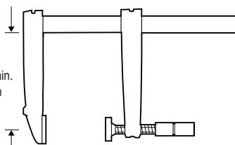
**Two heavy duty quick action or gripper clamps with throats of at least 100mm (4") are required to secure the jig to the worktop.**
