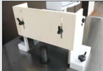
The optional tenoning hood is suitable for use with larger diameter tools (up to 300mm diameter); particularly tenon tools for producing doors.
