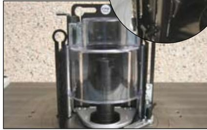
The ring fence comes as standard with the machine and replaces the back-fence when producing curved and circular work. It comes complete with adjustable guarding, lead on finger and a 100mm diameter dust extraction port.
