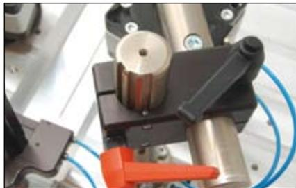
The indexed clamping toggle makes it easy to adjust the Archpress to suit different wood thicknesses and widths. You can also set the angle of the clamping cylinders.
