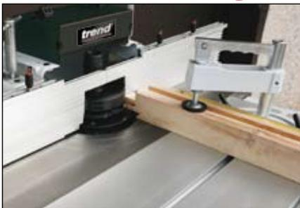
The aluminium flush mounted table runs on 8 high precision bearings ensuring smooth running and outstanding accuracy. A slot in the table is used for locating the tenoning clamp or the optional Tenoning Table.
