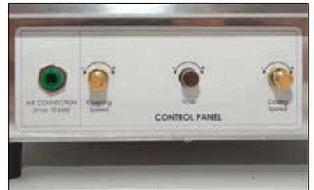
The main switchboard allows you to independently adjust the opening and closing speed and also set the clamping time.
