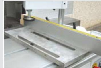
The 20mm thick tenoning table fits easily into the slot on the sliding table. Used in conjunction with the tenoning clamp and fence; suitable for getting smaller workpieces closer to the cutter heads.
