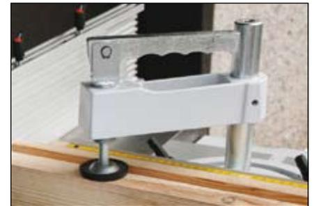
The eccentric clamp comes as standard with the machine and fits into the locating slot on the sliding table. It provides firm and positive clamping, essential when performing any tenoning operation.
