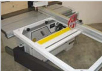
The optional table extension enables larger sections to be machined easily. Particularly suitable if you want to produce doors and larger windows.
