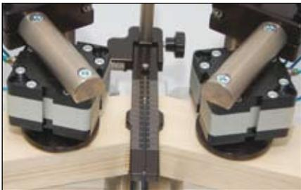
Adjusting the clamping height is simple. Just set the thickness of the wood on the laser marked scale and it's done.
