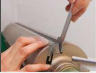
Tighten up the locking nuts.
