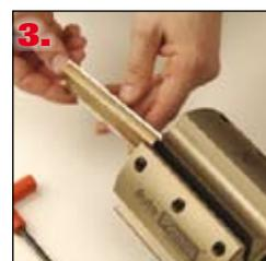
3. The cartridge is then inserted from the side...
