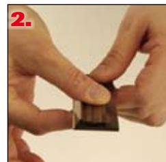
2. The knife is held to the wedge by the magnets. By pushing the wedge from the top, the knife can be easily and precisely positioned against the wedge.
