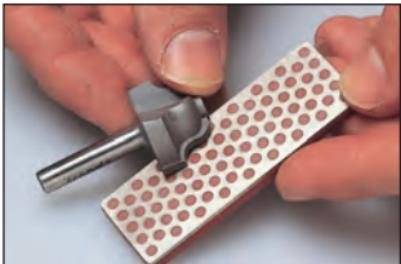
When honing your router cutters, apply light even pressure and use an equal number of strokes on each cutting face.
