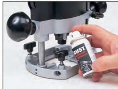
Rustbuster® is used to lubricate the pillars of the router & to prevent surface corrosion.
