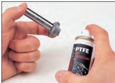
Regular application of a dry lubricant spray will prevent resin build up.
