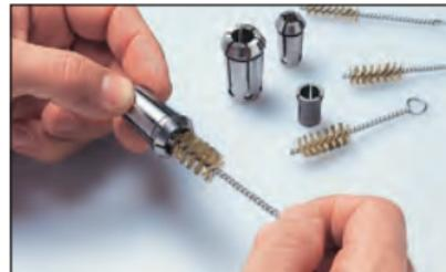
Brass brushes should be used to remove deposits from the inside of the collet.
