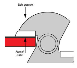
Ball-bearing guides should be removed from the cutter and care taken not to run the ball-bearing locating spigot against the stone. The latter is even more important for pin guided cutters, as marking the pin will effect its ability to run smoothly along the edge of the workpiece. Always ensure that the cutter is cleaned of all resin deposits, as this will be transferred to and clog the sharpening stone.
