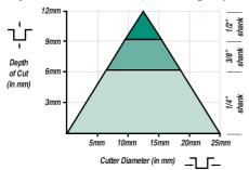
**Example:** Ref. 3/6 (10mm diameter cutter) For 1/2" Shank maximum depth of cut = 10mm For 1/4" Shank maximum depth of cut = 6mm
