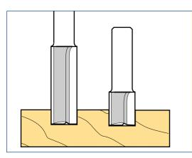
Whenever possible, use a cutter of a similar cutting edge length as the final depth of cut. As a general rule when using cutters below 6.3mm (1/4") diameter, on hard or abrasive timbers and materials, the cutting depth is best kept to no more than half the shank diameter.
