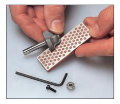
To hone the face of the cutting edge, press the flat face on the surface of the stone and ensure it is kept flat while drawing it back and forth along the edge several times. The amount of material removed will depend on the grade of the stone, so only use coarse stones if the cutting edges are particularly dull.
