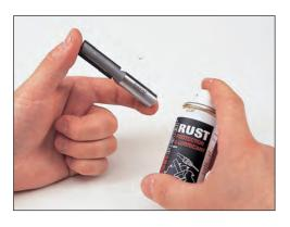
Before storing your cutters, apply an anti-corrosion spray such as Rustbuster®. This is particularly important if the cutters will be stored in humid conditions, such as in a shed or workshop, that suffers from excessive changes in temperature. This will prevent surface corrosion forming that will cause the cutter to bind in the collet. Be sure to keep spray away from the ball-bearing guide.
