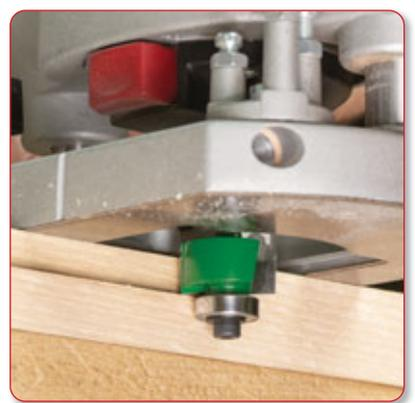
Ideal with delicate applications such as musical instrument production, when a small rebate is required for insertion of purfling.
