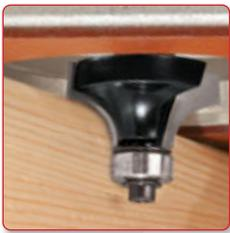
Rounding over a mould.
