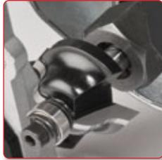
Ogee cutter fitted in a router.
