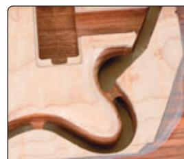
Tags holding mould workpiece in place.
