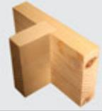
Through housing joint using tenon slide template.
