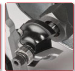
Ogee cutter fitted in a router.
