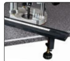
Long pivot clamp securing extrusion to worktop.
