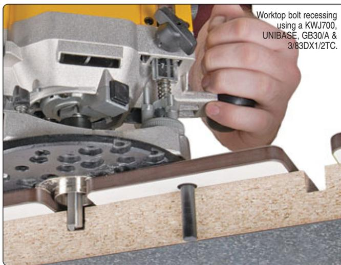
Worktop bolt recessing using a KWJ700, UNIBASE, GB30/A & 3/83DX1/2TC.
