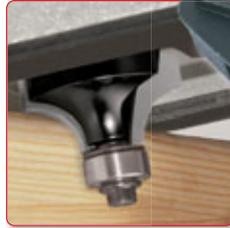
Rounding over a mould.
