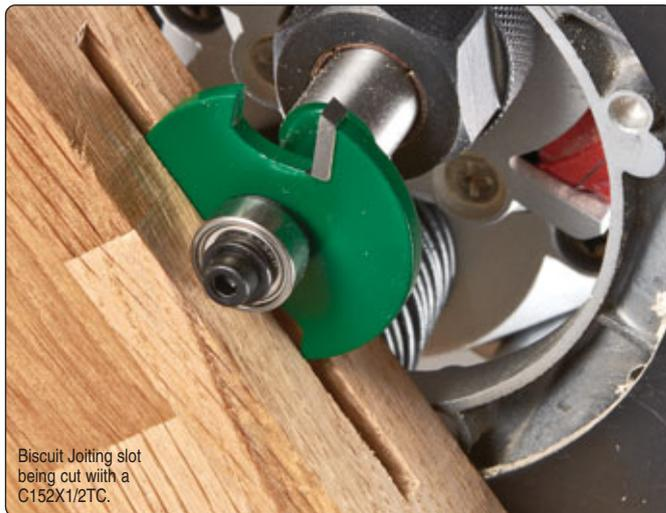
Biscuit Jointing slot being cut with a C152X1/2TC.
