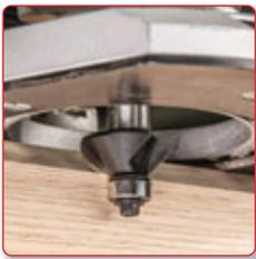
Rounding a chamfer.
