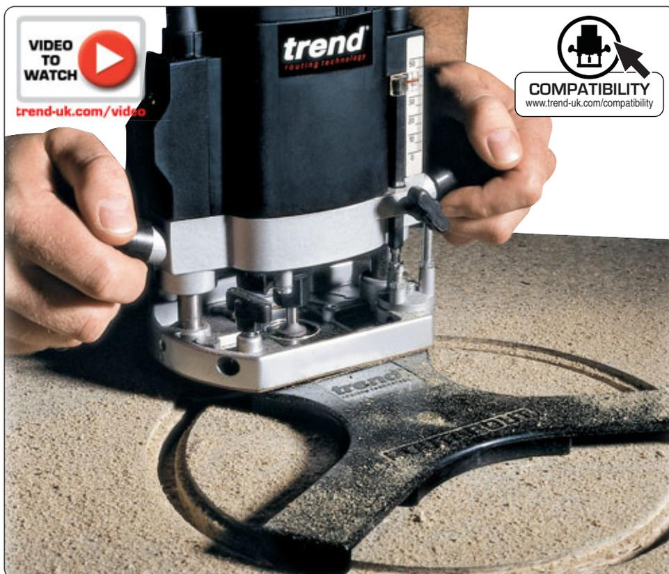
**Access to pipes and cables beneath chipboard floors in seconds. For builders, plumbers and electricians.**
