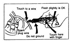
Note this check lamp does not light up very brightly because of weak electricity of atomospheric discharge from insulated spark plug wire.
