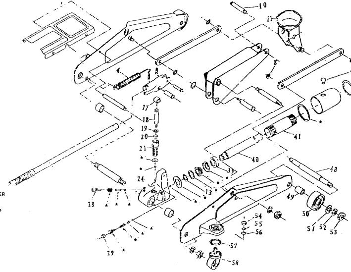
RETURN SPRING PIN, SADDLE HOLDER SADDLE ASS'Y RETAINING RING CLIP, PISTON, PUMP PISTON, PUMP O-RING SEAL ASS'Y CYLINDER BASE BASE RELEASE VALVE CAP, VALVE SPACER, RAM PLUNGER, RAM CYLINDER PLUG, FILLER FRONT AXLE BUSH, WHEEL WHEEL, FRONT WASHER LOCK WASHER NUT NUT LOCK WASHER WASHER BALL CASTER ASS'Y
