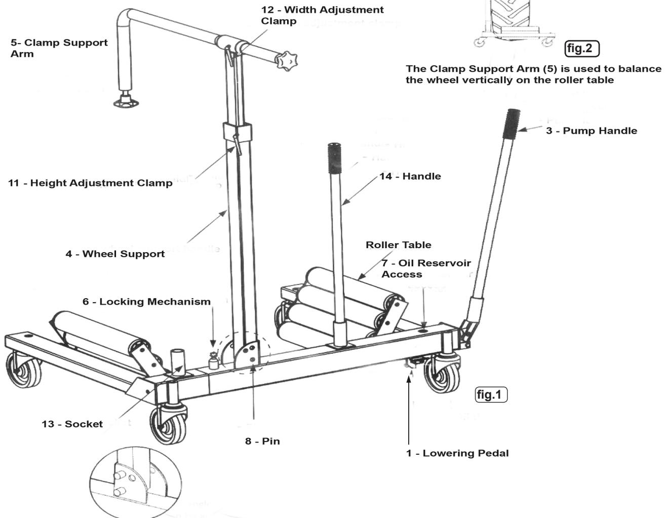
The Clamp Support Arm (5) is used to balance the wheel vertically on the roller table
