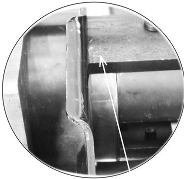
Segment edge flush with housing face, bush is now inserted to correct depth.
