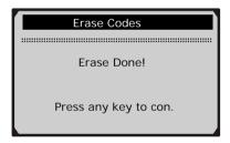
• If the codes are not cleared, then an "Erase Failure. Turn Key on with Engine off!" message appears.
