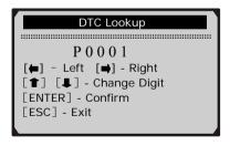
3) View the DTC definition on screen. When DTC definition covers more than one screen, use **LEFT/RIHT** button to view additional information on previous/next screens.
