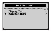
2) Press any key to start test. When you press a key, the key name should be observed on the display. If the key name does not show up, then the key is not functioning properly.
