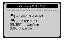
9) Use **RIGHT** button to deselect/select data parameters, and use **UP/DOWN** scroll button to move up and down. Selected parameters are marked with solid squares.
