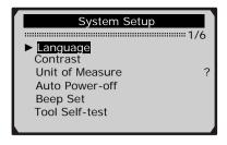
**From the Main Menu:** Use the **UP/DOWN** scroll button to select **System Setup**, and press **ENTER** button. Follow the instructions to make adjustments and settings as described in the following setup options.
