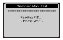
3) From **On-Board Mon. Test** menu, use **UP/DOWN** scroll button to select a test to view and press **ENTER** button.
