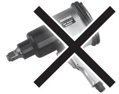
The force screw maximum recommended torque is 170Nm (M18x1.5), 155Nm (M16X1.5), 99Nm (M14X1.5), 60Nm (M12X1.5), 33Nm (M10X1.5). Exceeding these torque values may shorten the life of the force screws. The force screws are considered to be consumable items and are NOT covered under warranty.
