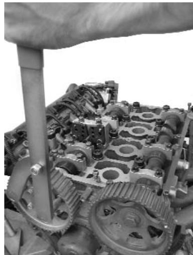
**WARNING: DO NOT use Al-Fi Camshaft Setting Plate Assemblies to counter-hold camshafts in position whilst releasing or tightening the sprocket bolts as this will damage the Setting Plates. Al-Fi Assemblies are for retention of timing position only. A suitable Sprocket Holding Tool MUST BE used to counter-hold the sprockets.**
