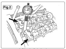
Left-hand cylinder head Camshaft Setting Plates location (viewed from camshaft sprockets)
