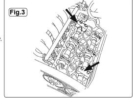
Right-hand cylinder head Camshaft Setting Plates location (viewed from camshaft sprockets)
