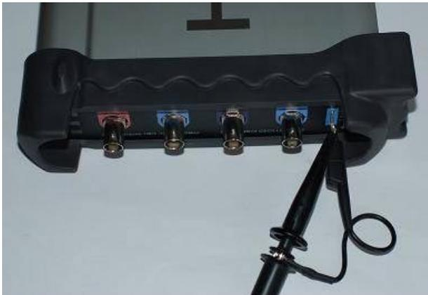
2. Set the CH1 probe attenuation of the oscilloscope to x10. (The default is x1).
