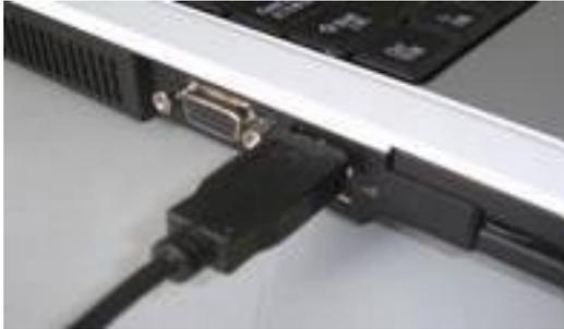
2. Connect the B-Type Plug of the USB cable to the **TA4000** USB port.
