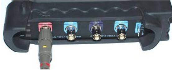
**CH1/CH2/CH3/CH4:** Input connectors for waveform display.
