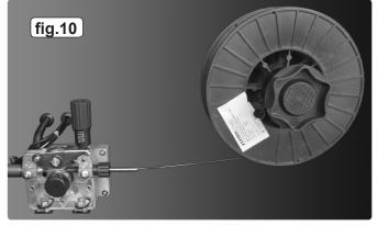
3.9 FEED WIRE THROUGH TO TORCH. Referring to fig.12 open the wire feed mechanism by pushing the locking/wire tension knob (1) down to the right allowing the pressure roller carrier (2) to spring up revealing the feed roller. Ensure that the required feed groove (0.6 or 0.8) is in line with the wire path. See Section 3.12 on how to reverse or change the roller.
