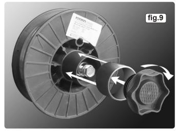
3.8 FITTING A 5KG REEL OF WIRE. Ensure that the wire diameter used, is matched by the correct groove size in the drive wheel and the correct tip size on the torch as well as the correct torch liner. Failure to do this could cause the wire to slip and/or bind.
