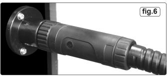
3.6 CONNECT THE TORCH CABLE TO THE WELDER. Align the pins on the Euro connector with the socket on the welder front panel as shown in fig.5. Push the connector into the socket and rotate the locking ring (A) clockwise so that it draws the plug into the socket as shown in fig.6.
