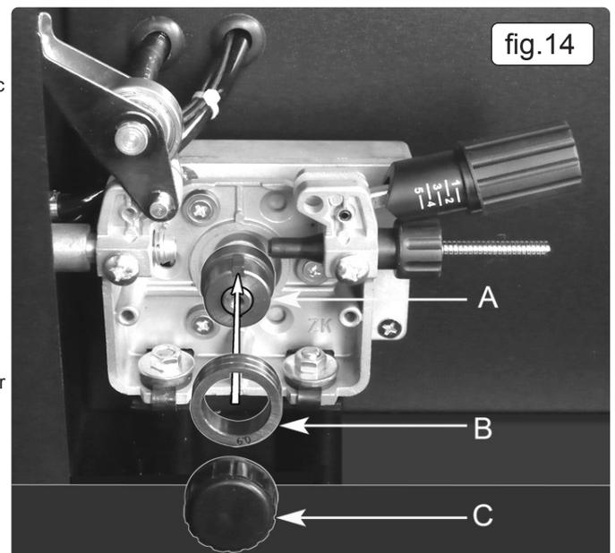
Ensure that the wire diameter used, is matched by the correct groove size in the drive wheel and the correct tip size on the torch as well as the correct torch liner. Failure to do this could cause the wire to slip and/or bind.
