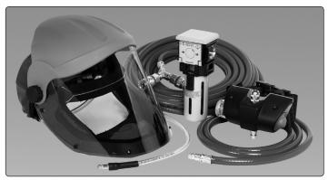
The SSP201K system comprises a lightweight mask connected via a breathing hose to a pre-set regulator, with spare carbon filter, mounted on a comfortable waist belt with quick release buckle. The hose kit consists of a compressed air supply hose and couplings, fitted with a "Y" piece which connects to the pre-set regulator. A 1.5 metre compressed air supply hose is provided for connection of a spray gun. A wall-mounted coalescing filter is supplied in the kit.
