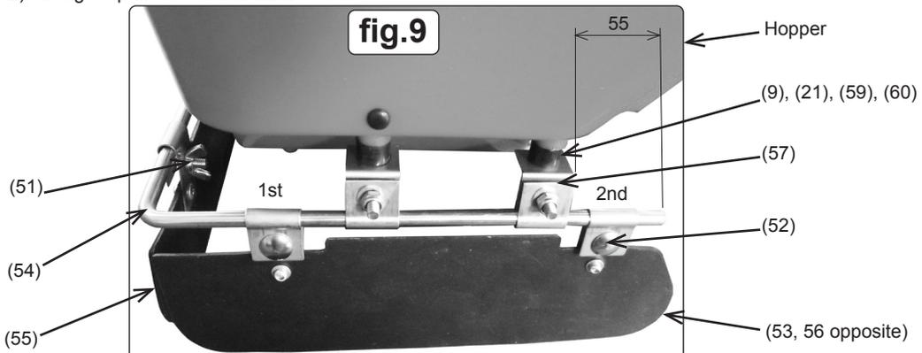
**5.7. Refer to fig.9 for fitting front and side deflectors.**
