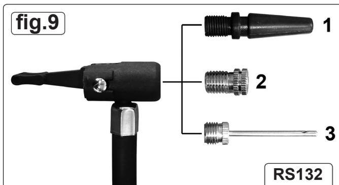
7.2.3. Identify the correct adaptor for the product and insert it into the inflation connector as indicated in fig.9 and push the locking lever through 90° to lock it.
