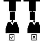
Piston rod should face workpiece
