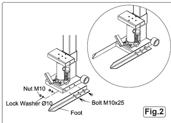
3.1.3. Attach the two feet to the bottom of the main post. Secure each foot using two M10 bolts, two lock washers Ø10 and two M10 nuts. Bolt through the two outer holes (fig.2).
