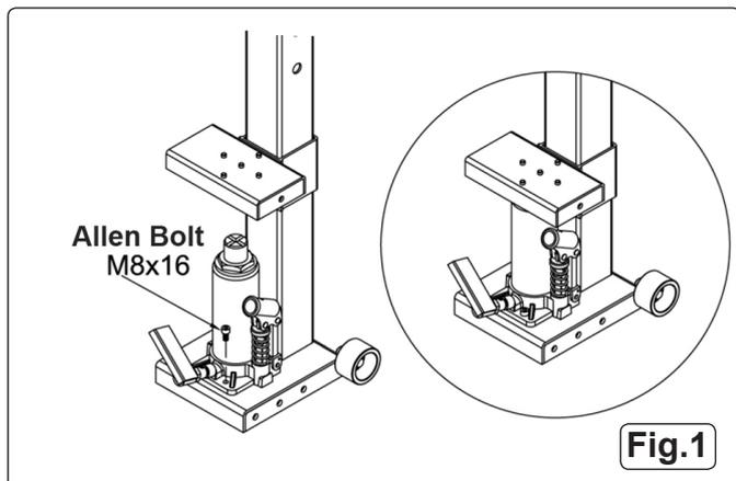
3.1.2. Slide the log support over the main post and down onto the hydraulic pump unit (fig.1).
