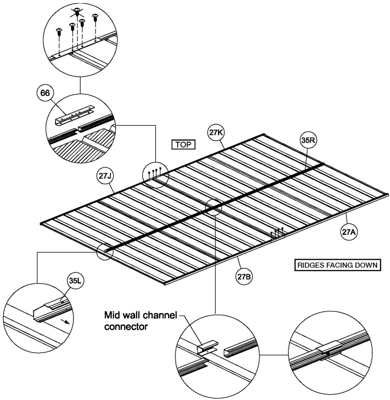
**Step 4:** Assemble the roof panels
