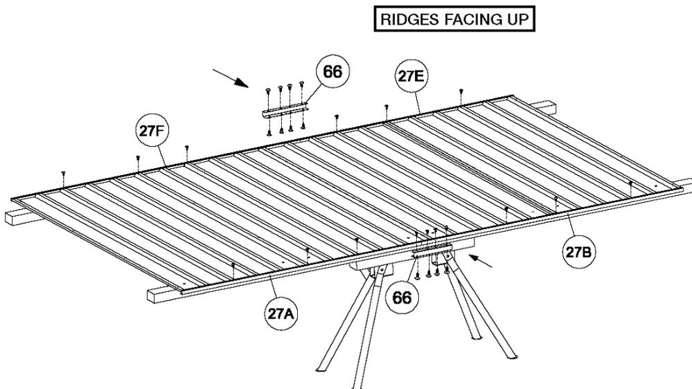
Enhance the structural strength by applying part 66 (channel connectors). Note that screws are applied to both sides of the connectors as per Step 3.
