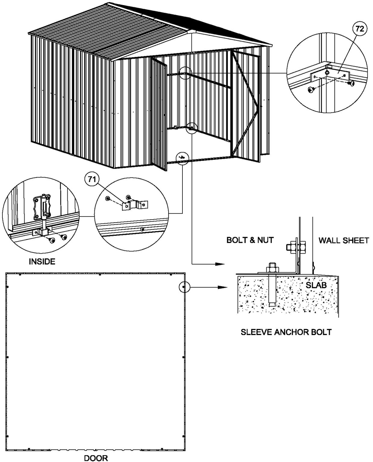
Apply channel safety cover L type to channel 33L and R type to channel 33R for safety. Also apply the self-tapper covers to the screw ends visible in walls on the inside of the shed.
