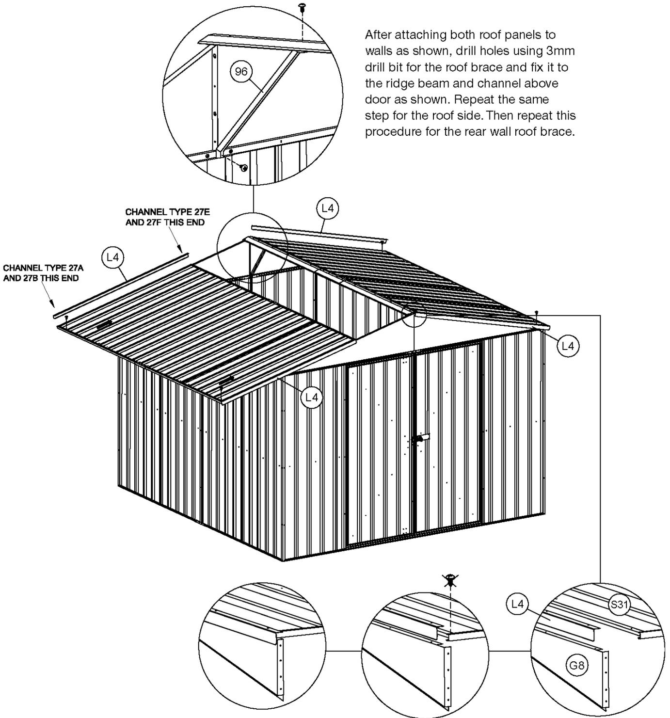
After attaching both roof panels to walls as shown, drill holes using 3mm drill bit for the roof brace and fix it to the ridge beam and channel above door as shown. Repeat the same step for the roof side. Then repeat this procedure for the rear wall roof brace.
