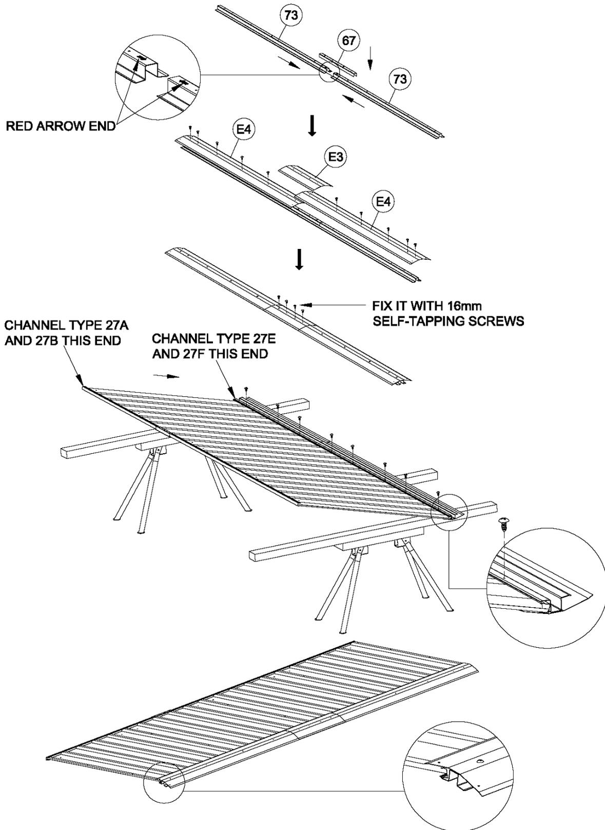
Slide the side of the roof panel with channels 27E and 27F into the ridge beam.
