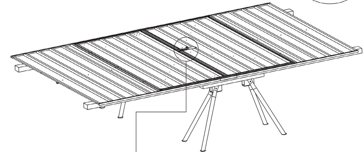
FIX PADBOLT KEEPER WITH 16mm SCREWS
