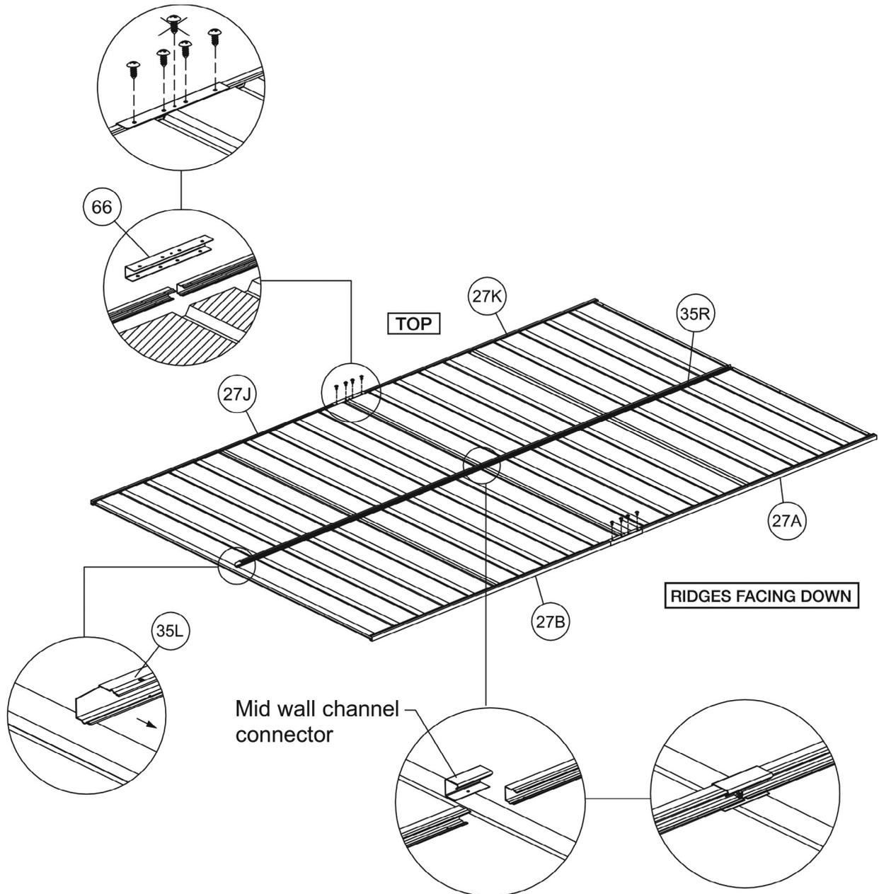
**Step 4:** Assemble the roof panels
