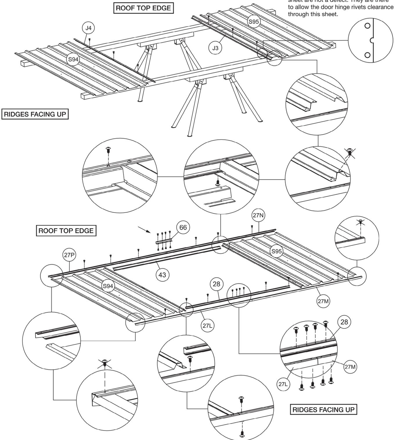
Fix parts 27P and 27N (top channels), part 43 (jamb), and parts 27L, 27M, and 28 (bottom channels) using self-tapping screws. Enhance the top channels by applying part 66 (channel connector) and fix screws through both sides. Please note: for parts 27P, 27N, 27L and 27M the small lip should be facing out to stop water building up and leaking into shed.
