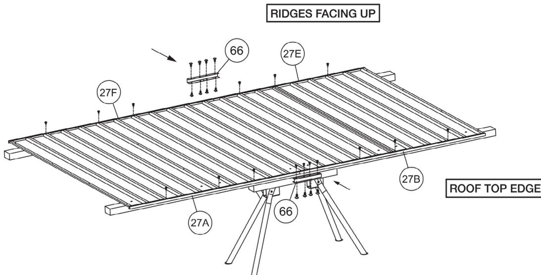
Enhance the structural strength by applying part 66 (channel connectors). Note that screws are applied to both sides of the connectors as per Step 3.
