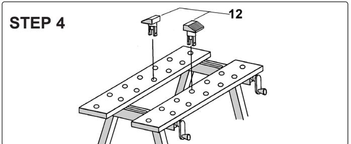
Fix chock (12) in suitable holes located in worktop as required.
