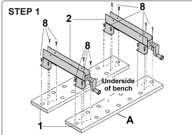
Lay the wooden worktop/jaws (1) upside down on a surface that will not scratch or cause damage. Screw the slide bases (2) to the jaws using wood screws (8) ensuring that the jaw angle and ruler guides are on the same side as the vice handles at point "A".
