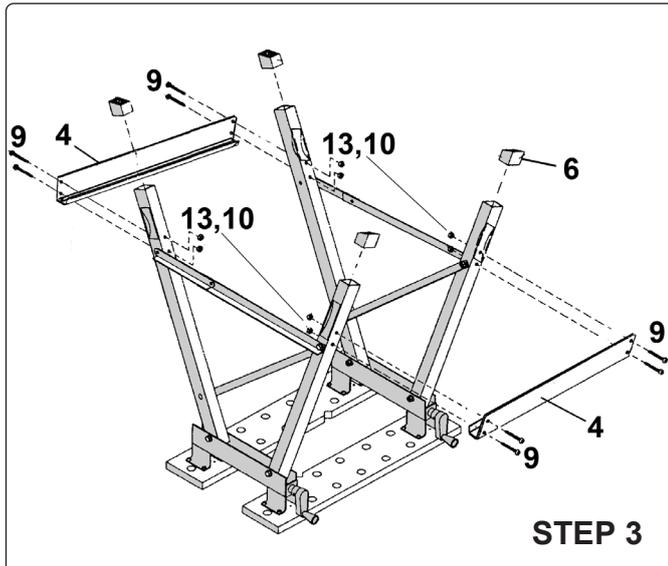
Align the crossbars (4) with holes in legs and insert screws (9) from the outside and fix with washers (13) and nuts (10).
