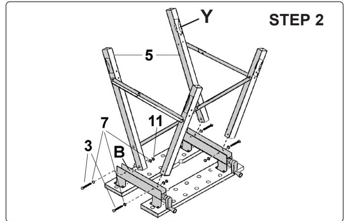
Open the leg frames (5) and align with holes on the inside of the vice arms at points "B" ensuring the curvatures on the lower part of the legs "Y" point outward. Insert bolts (3) from the outside of the vice arm with washers (7) and secure with washers (7) and nuts (11) from the inside.
