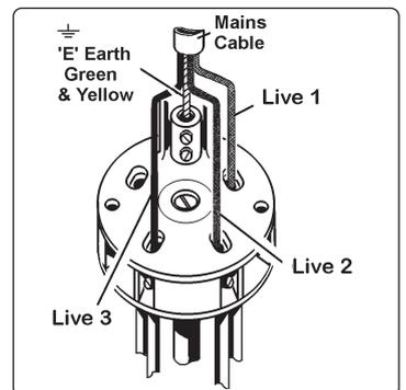
When completed, check that there are no bare wires, that all wires have been connected correctly, that the cable external insulation extends beyond the cable restraint and that the restraint is tight.
