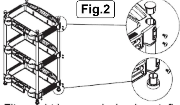
Fit upright inner and wheel seat, fix screws (3/16 x 1/2") on each seat.
