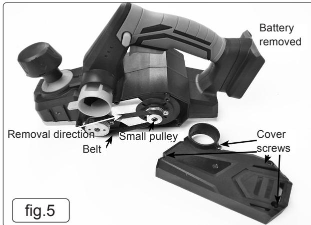
**NOTE:** When replacing the belt, use the recommended Sealey replacement belt only.
