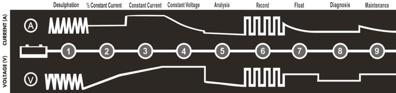
Stage 1: Desulphation: Pulses of current and voltage.
