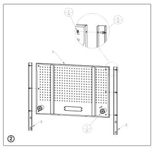
**Step 2**. Insert the supplied Screws and Locking Nuts – Drive screws through the Support Pillars into the Pegboard, as shown in the above illustration making sure they are tight. Insert the 2 Plastic Grommets as shown.
