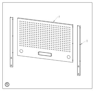
**Step 1**. Align the Pegboard 'A' and Pegboard Support Pillars 'B' – Hold the pegboard against the Support pillars, ensuring the pre-drilled holes align.
