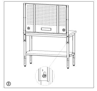
**Step 3**. Align the Pegboard 'A' assembly up with the back of bench. Align the predrilled holes and screw the pegboard to the bench as illustrated. Tighten bolts to finish.
