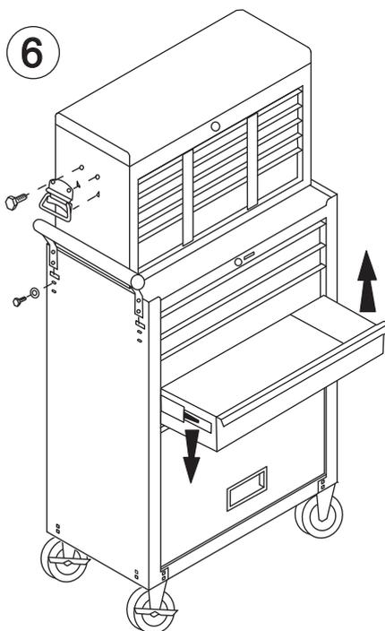
To remove a drawer, pull the drawer completely out, press down the left tab and lift up the right tab, pull drawer off the slides. To reinstall the drawer, realign with the internal drawer slide and push until it locks in place.
