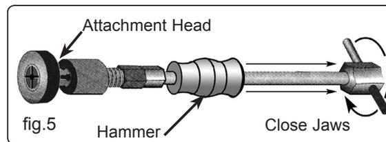
5.8. Turn the handle anticlockwise to close the jaws in order to release the bearing from the attachment head. See fig.5.
