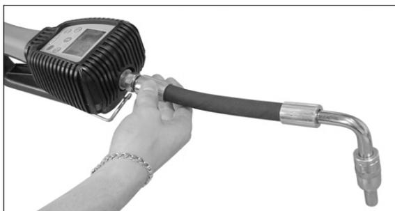
Installing the nozzle
