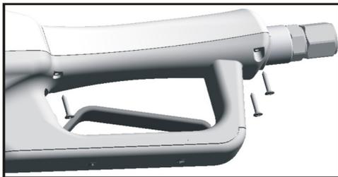
6.1.2 Open the battery pack by removing the cover.
