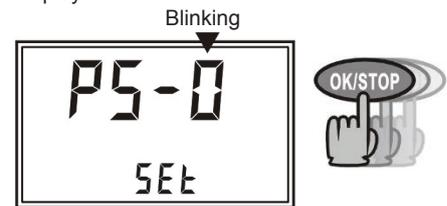
4.9.2 When PS factor is blinking, press **AUTO** to select PS 0-4 to increase the PS factor by one unit.
