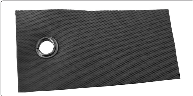
4.6. Underside of finished eyelet.
