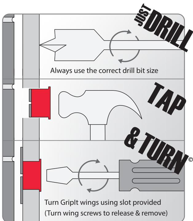
1. Mark out the centreline positions where GriplIt fixings are to be installed, then drill the required number of holes in the plasterboard. We recommend using a GriplIt hole cutter or a flat drill bit. (see [www.griplitfixings.co.uk/accessories](http://www.griplitfixings.co.uk/accessories))
